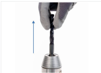
Fig. 8: Remove the tool
