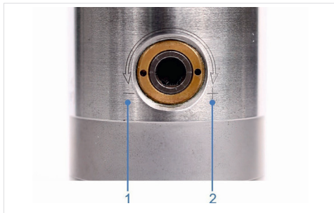
Fig. 3: Indication of the direction of rotation for clamping and unclamping the tool
