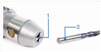
Fig. 4: Cleaning precision drill chuck and tool
