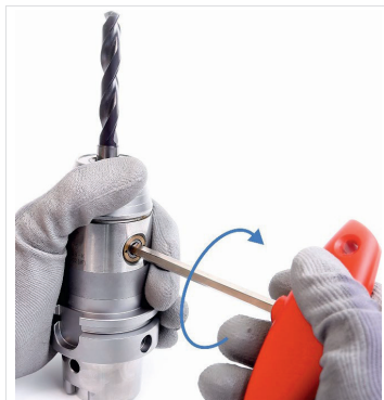
Fig. 6: Clamp the tool
